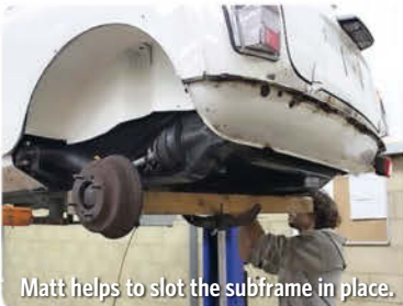
Inner arches were primed and repainted.
