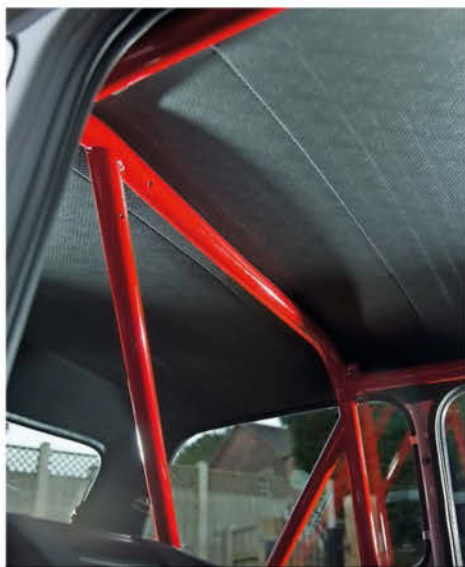
Colour-coded 'cage sits below a black perforated headlining, which Steven says was a difficult fit.
