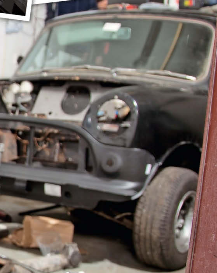
Inner wings were removed to fit a Vauxhall 16-valve motor.
