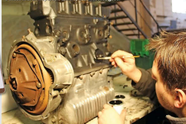
Kevin at Sussex Road and Race gave the engine's bores a check with an inspection camera, and all looked good.
