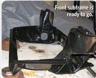
Suspension parts nicely coated in POR15.
